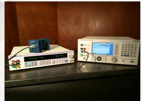
The AC/DC shunts consist of a total of 14 high precision shunts, each with an output value of 0.7V for full scale nominal input. These shunts come in various input values of the following values
