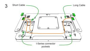
Remove the connector covers from each status light and connect the GPIO cables as shown. Use the short cable to connect the nearest light to the I-Series GPIO connector. Use the long cable to connect a second light to the first light. Then reinstall the connector covers making sure the cables route through the openings in the covers and are not pinched.
