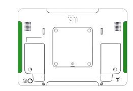
Remove the Edge Connect peripheral covers to expose the peripheral bay. Up to two status lights can be installed on a single I-Series display
