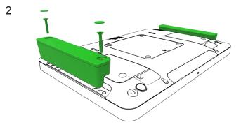
Gently press the status light into the Edge Connect peripheral bay making sure the connector is seated. Then install the included screws and screw covers.
