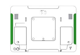
Remove the Edge Connect peripheral covers to expose the mounting interface. Up to two status lights can be installed on a single I-Series display
