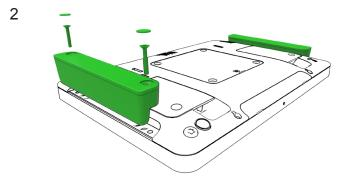
Fasten the status light to the I-Series using the included screws and screw covers.
