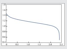
The built-in battery test function uses CC mode to calculate the battery capacity using a fixed current load discharge. Users can specify cut-off voltage level, capacity level and time stop conditions.
