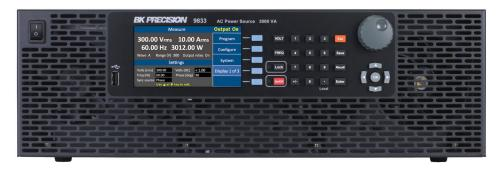
The 9830 Series are low distortion, single-phase AC power sources delivering a maximum of 3000 VA, 300 Vrms, 30 Arms / 97.5 Apk with the output frequency adjustable from 45 Hz to 1200 Hz. Housed in a compact 3U form factor, the AC source is capable of generating both AC, DC, and AC+DC output.
