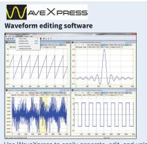
Use WaveXpress to easily generate, edit, and upload custom arbitrary waveforms to the generator via the remote interface. Generate waveforms in the software by importing a text file or define via freehand, point draw, and waveform math functions.
