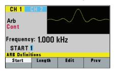
From the front panel, waveforms can be defined from scratch by entering data point-by-point or by loading and modifying predefined waveforms.
