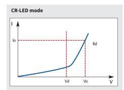
Use the load's unique CR-LED operating mode to test LED drivers. This function allows users to configure the LED's operating resistance and forward voltage to simulate the loading behavior of typical LEDs.
