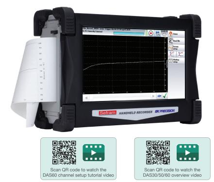
The DAS30/50/60 high-speed multi-function recorders are suited for motor monitoring, manufacturing, and industrial applications. They feature 2, 4 or 6 configurable channels, high-speed sampling (1 MSa/s), a wide input range (±5 mV to ±500 V), large internal solid-state memory up to 64 GB, 9.5 hrs of battery life, and CAT III isolation rating.
