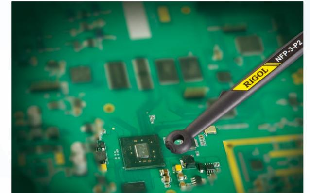
NFP-3-P3, a near-field probe which resolution is 5 mm. It is applicable for the detection magnetic field on surface. For example, the detection of the magnetic field produced by the wire, cable, metal surface, connectors, electronic components, and component joints.
