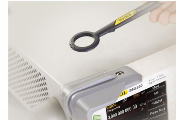
NFP-3-P2, a near-field probe which can detect the magnetic field within a range of 3 cm. It is applicable for detecting the magnetic environment around the modules. For example, accurately locating the leakage of the chassis, detecting the magnetic field direction and intensity of the circuit board module.
