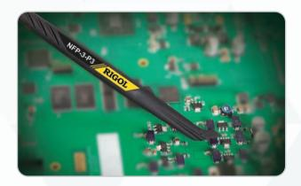
NFP-3-P3, a near-field probe which resolution is 5 mm. It is applicable for the detection magnetic field on surface. For example, the detection of the magnetic field produced by the wire, cable, metal surface, connectors, electronic components, and component joints.
