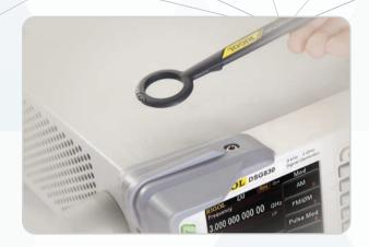
NFP-3-P1, a near-field probe which can detect the magnetic field within a range of 10 cm. It is applicable for the leakage detection of magnetic field. For example, verification of shielding measurement, leakage testing for the chassis etc.
