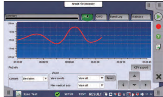
Phase Confirmation using MU100090A
