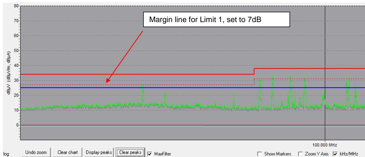
By default, the margins are set to 0, so any peak crossing the limit line would be indicated. Setting margin1 to e.g. 7dB would select all peaks coming within 7 dB close to the limit line of the graph measured with Settings1. Peaks crossing the margin line or limit line can be listed in the in the **Peaks window** by pressing the **Display peaks** button.
