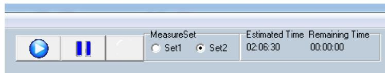
Most project files define Peak or Average measurements as Set1 and Quasi-Peak measurements as Set2. By default, all segments are measured and displayed consecutively.
