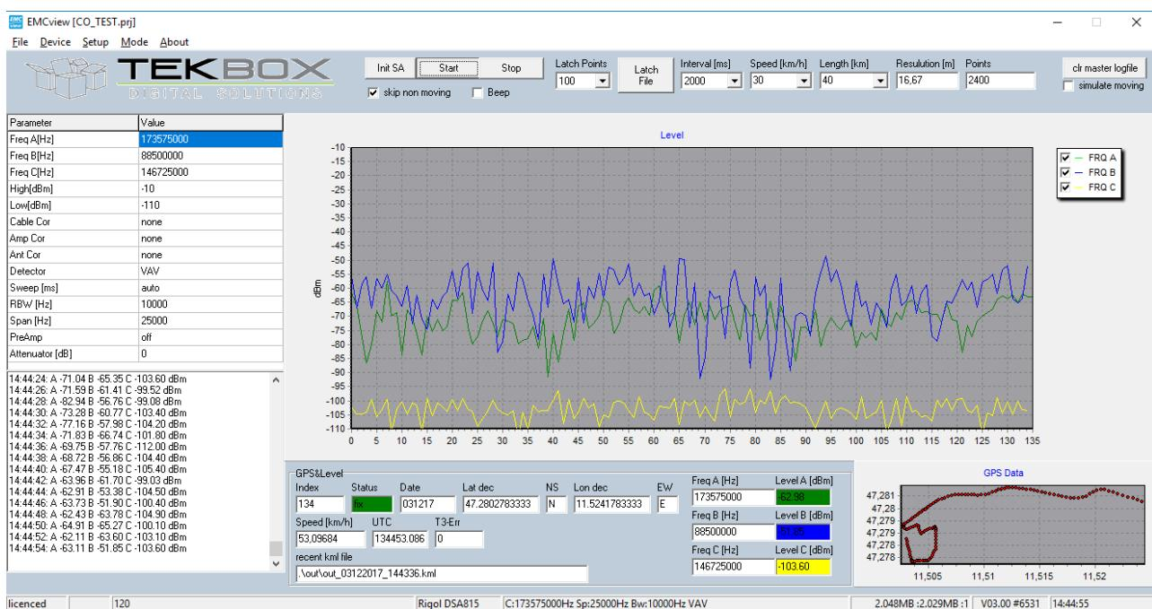
The main graph displays the measured field strength of the observed transmitters on the y- Axis and the index number of the corresponding measurement on the X-axis.
