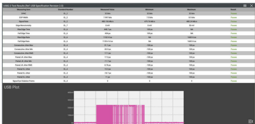
Figure 18.2 USB2.0 Signal Quality Compliance Analysis Test Result
