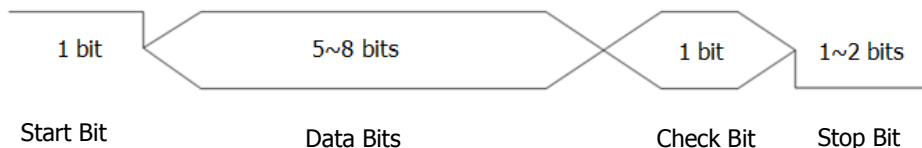
Figure 5-13 Schematic Diagram of RS232 Protocol
