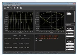
6. Click the symbol display area. Then, the symbol setting is displayed at the right section of the interface. You can select "Binary" or "Hex" as the display format of the symbol. You can also select "ON" or "OFF" to determine whether to display the symbol in Manchester encoding.
