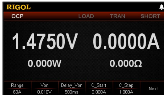
Figure 2-30 Main Interface of OCP Test Function
