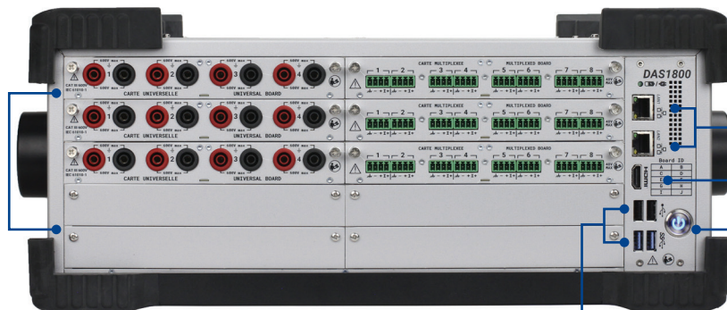
Image displays a DAS1800 configured with 3 universal modules and 3 multiplexed modules.
